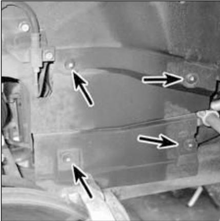
**22.2** Remove fasteners from the front of the inner fender liner and pull it back for access (see Chapter 11), then remove this splash shield from the right fenderwell to gain access to the drivebelt tensioner (two rear pushpins not visible in this photo)
