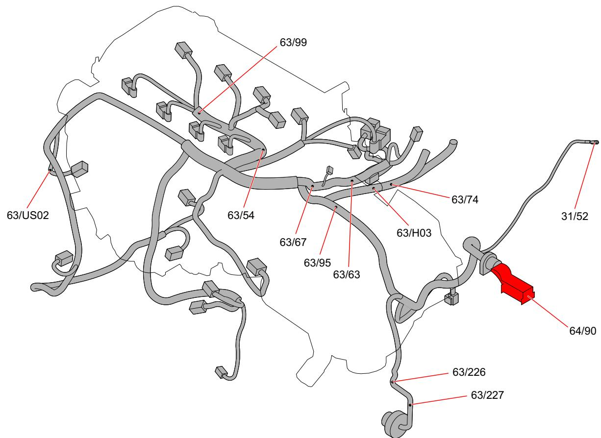
Cable harnesses' routing in the vehicle
