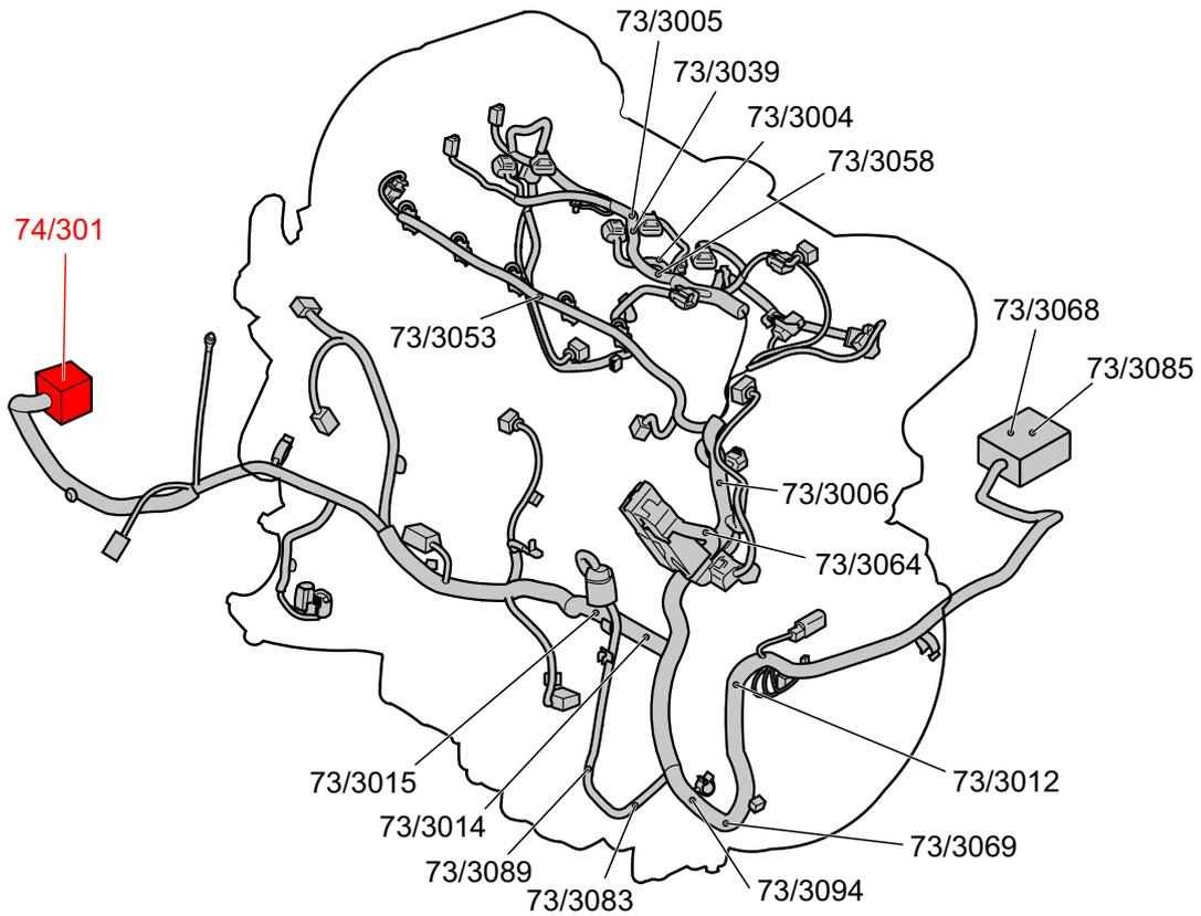
**Cable harness routing in vehicle**
